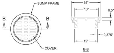
TYPICAL SUMP FRAME AND GRATE DETAIL
