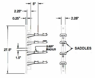
NOTE: FASTEN BY MEANS OF 2.5" X 0.5" BOLTS AND EXPANSION SHIELDS
