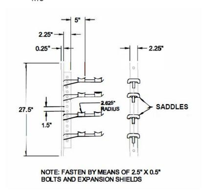
DETAIL B - CABLE RACKING
